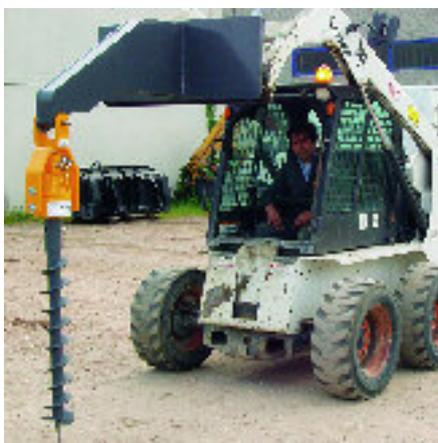
The new **UT** Series connection plate allows the auger drive unit to be attached and used on a skid loader.
